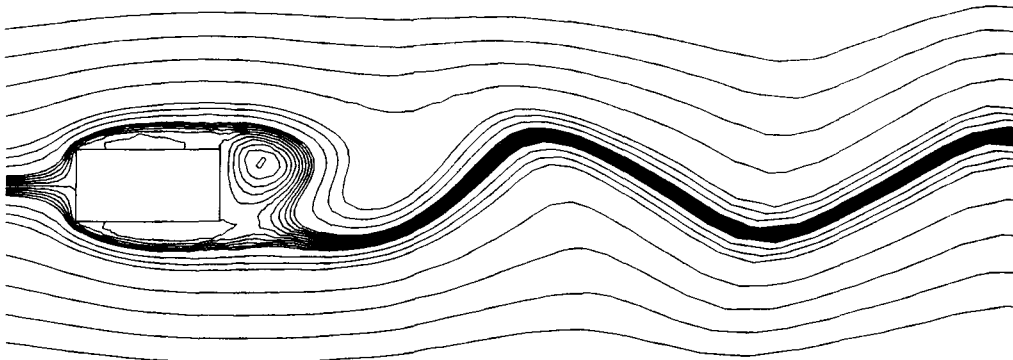
Figure 11. Plot of instantaneous streamlines near the obstacle at Re = 300 (mesh RECT2, \Delta t = 0.25 , two-step scheme, \beta linear)
